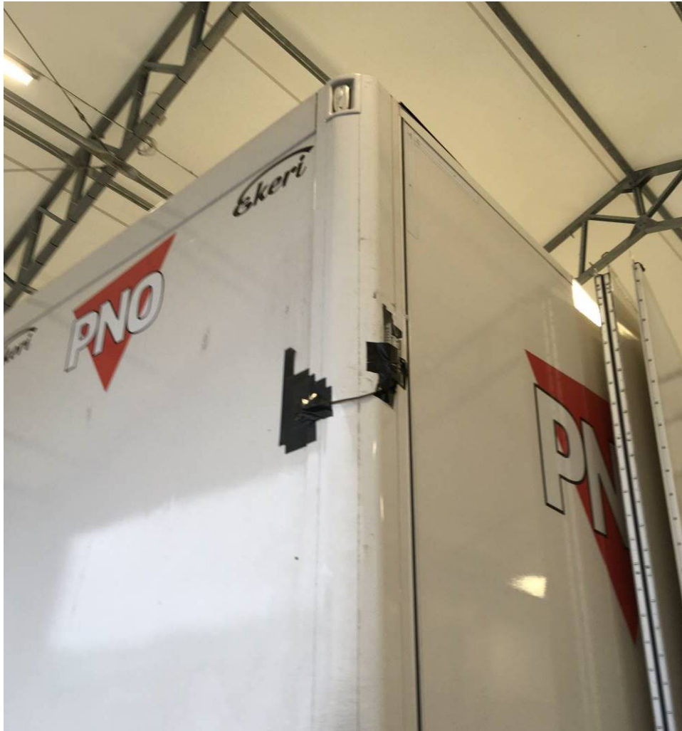
Photo 3: Ambient temperature sensor installation.
