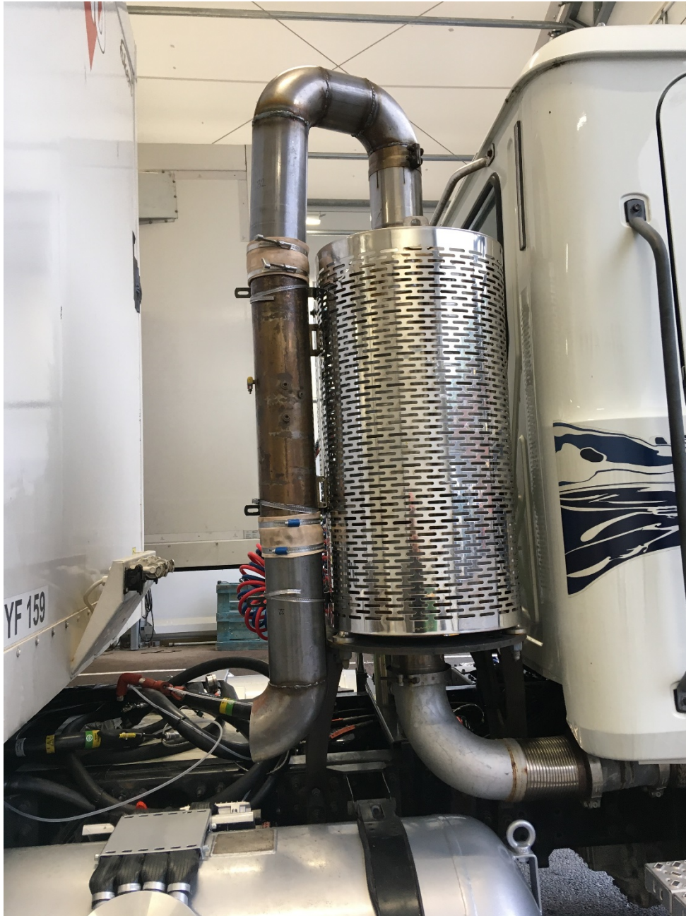
Photo 2: Exhaust system with EFM and sampling points
